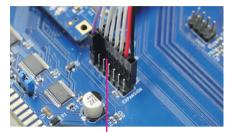
Connect the second half (7 pins) and the single purple lead of Data Cable to the EXPANSION header on ZZ9000 as pictured. Black and red go near the EXPANSION label.
