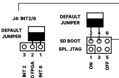
'J4: Interrupt select. Connects either Amiga interrupt INT2 or INT6 to the FPGA. Leave the jumper on INT6 to use Ethernet.
